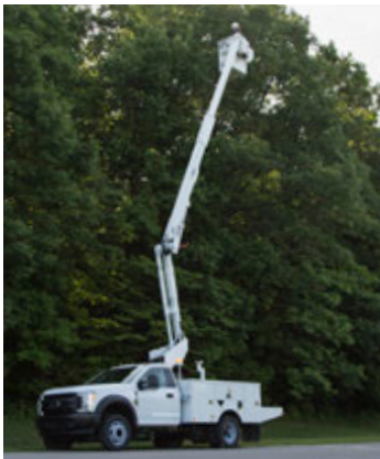
INCREASED WORKING HEIGHT 45.6 FT (13.9 M)
