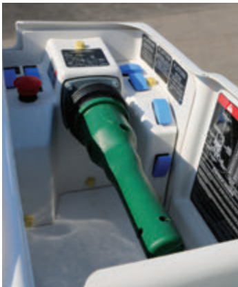
FIBER OPTIC CONTROLS WITH FEWER HOSES AND VALVES
