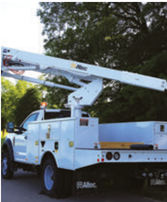
ISO-BOOM OPTION FOR ADDED DIELECTRIC INTEGRITY
